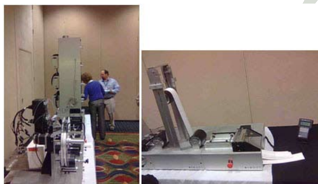
The In Line Web Handling System RR4500 with antibody dispensing module, dip tank, dry tower and enclosed take up module (right) were displayed during practical session. The BioDot workshop was a mixture of lectures and laboratory sessions where scientists reviewed the entire process of lateral flow applications.
